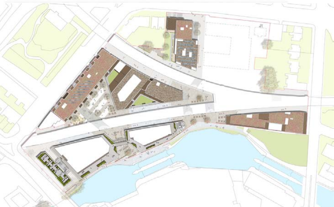
Roof masterplan, showing mixture of green and brown roofs prepared by Fabrik
