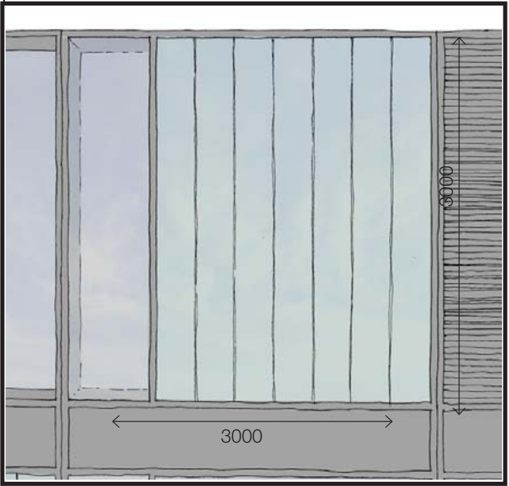
Curtain wall panel type B With a clear pane and vertical cast glass channels
