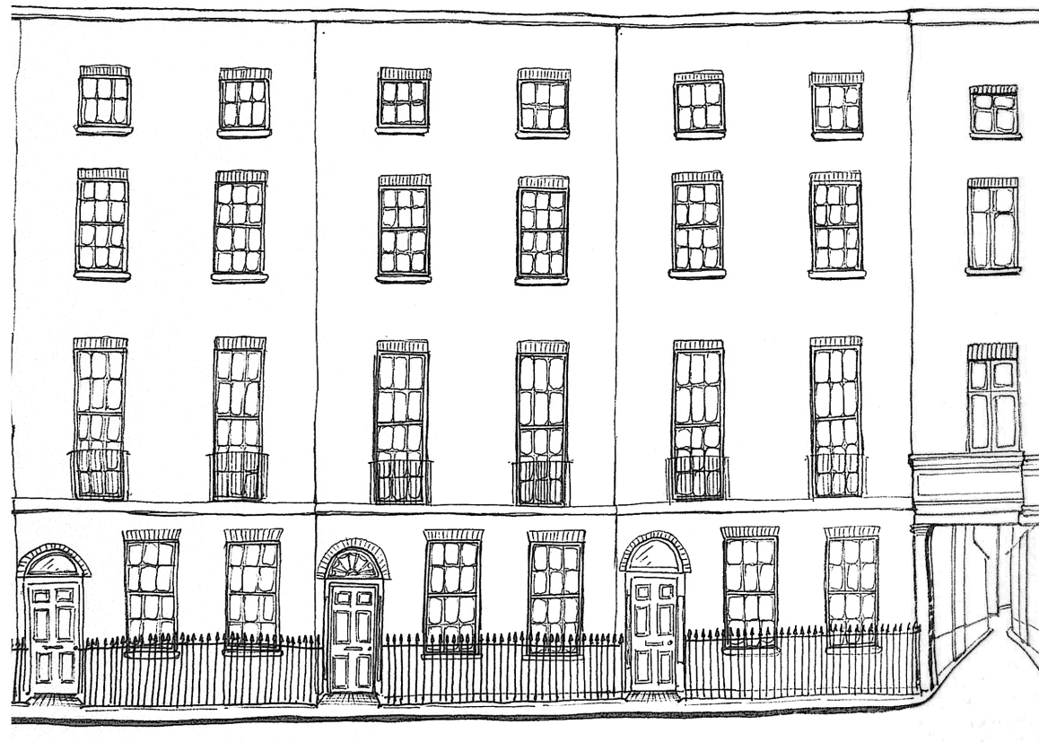
Fig. 05 A sketch demonstrating the front facade of No. 6 Conway Street, showing the six over six sash windows, which we intend to restore to their original splendour.
