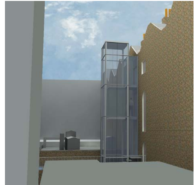
View to rear looking east showing minimal glass cladding system wrapped around the internal steel support for the lift. See page 26 for images of installations showing the intended quality of detailing and appearance.
