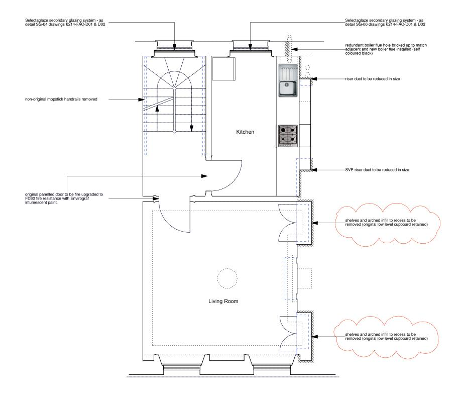
REV A (23/10/12) - proposed secondary glazing omitted to front room windows and chimney recess cupboard notes revised
