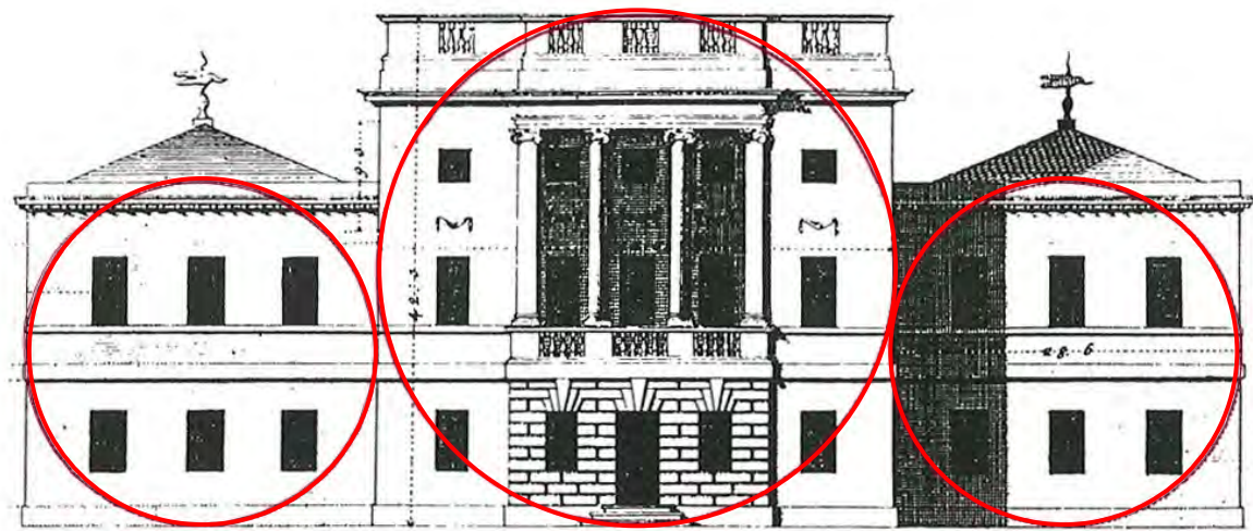
Palladian height to width facade proportion
