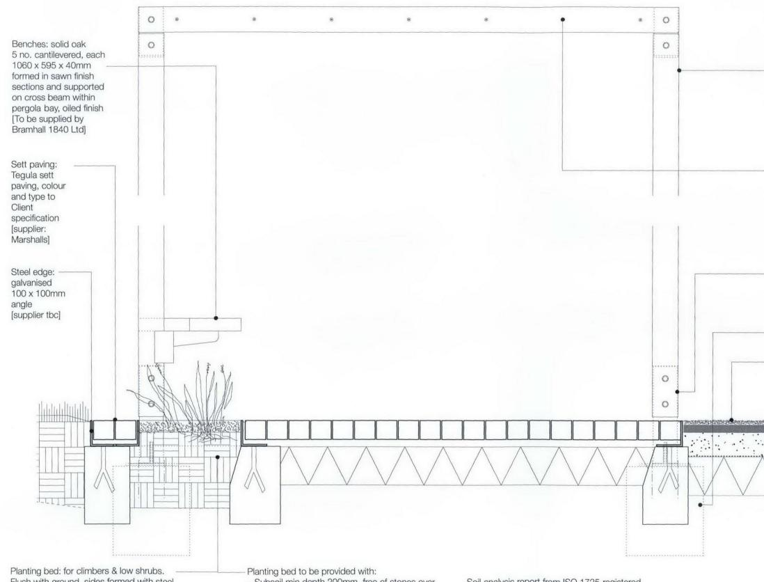
Flush with ground, sides formed with steel edge galvanised 100 x 100mm angle. Base to be open to the ground, free-draining and free of hardcore, brick, concrete, metal and extraneous material.
