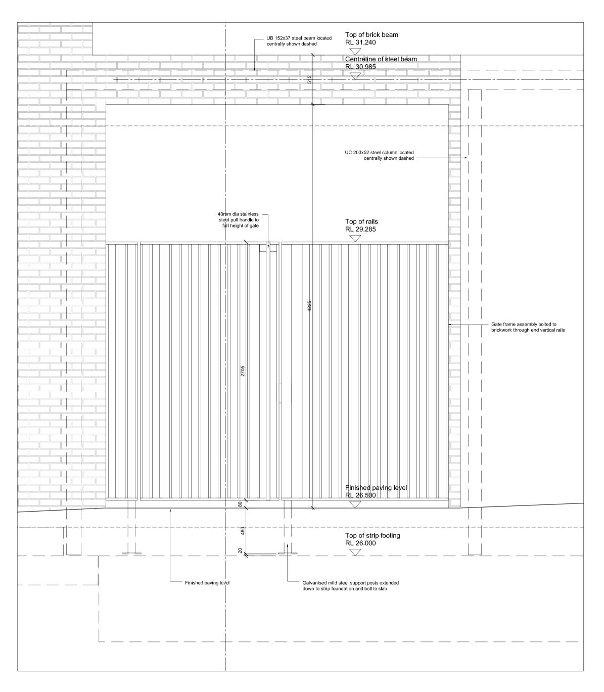
Elevation screen type 4 Scale: 1:20
