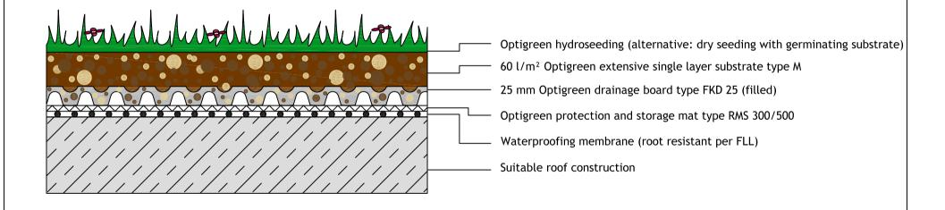
The depicted product solution is intended for use with green roof systems. Other construction tradework is simplified in this representation and should be constructed according to current industry standards. This drawing is not to scale. Optigreen reserves the right to make changes to its product solutions.
