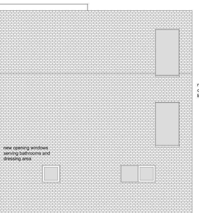
new fixed window openings allow light into internal stair
