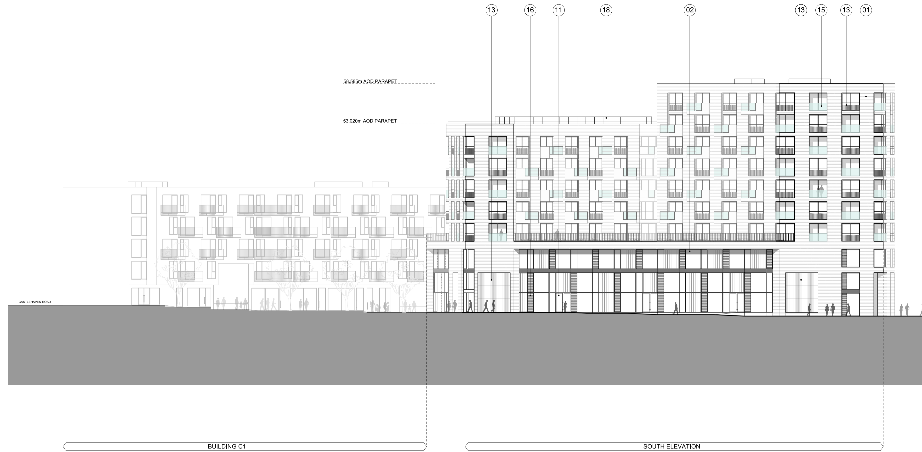
01 BUILDING C2_ SOUTH ELEVATION
