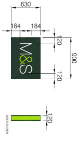
SIGNAGE TO HAVE LETTERING FACES IN OPAL ACRYLIC 5MM 050 & LIME ACRYLIC 5MM 6T84. FLUSH FACE WITH METAL USING EXACT DETAIL SHOWN ON THE GENERIC DRAWING.
