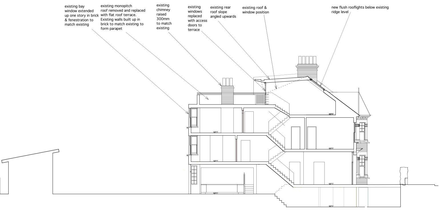
do not scale - check all dimensions on site 26 HOLMDALE ROAD LONDON NW6 1BL PROPOSED SECTION AA 4 M
