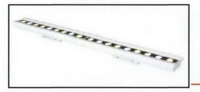
TYPE T1: Linear Led recessed in horizontal fin TRAXON HB Linear Shield XB DW Cool White 6500K, 105lm/W, IP66-rated DMX controlled including dimming. 27 high intensity power LED's
