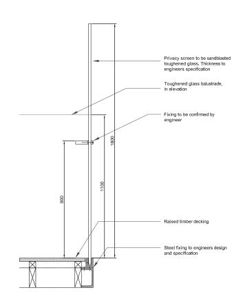
Section A Ground Floor / First Floor
