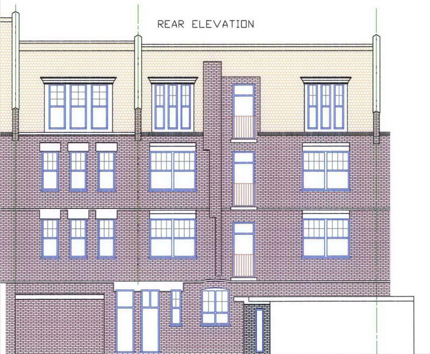
EXISTING REAR ELEVATION
