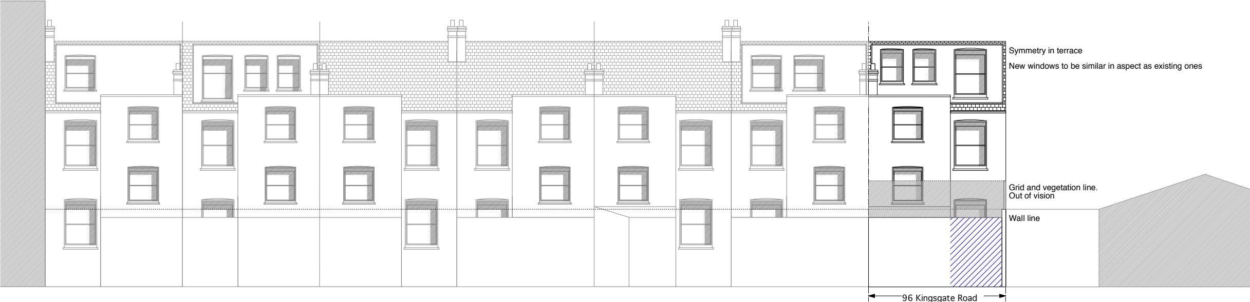
2 106 Elevation : Rear Elevation : Proposed Scale: 1:150 @ A3
