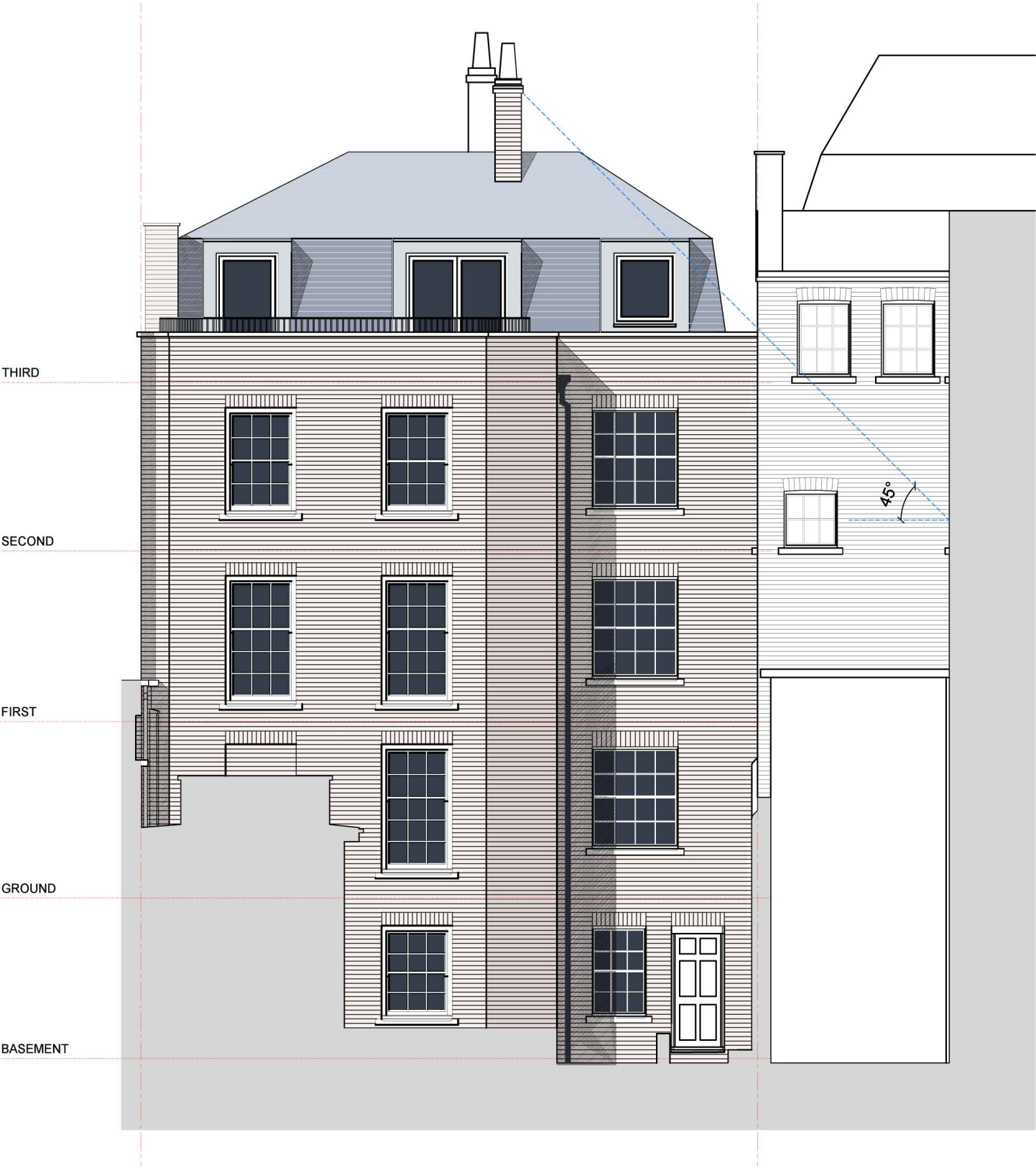
Proposed rear elevation indicating revised timber sash windows, removal of external terraces and modified treatment to the roof terrace
