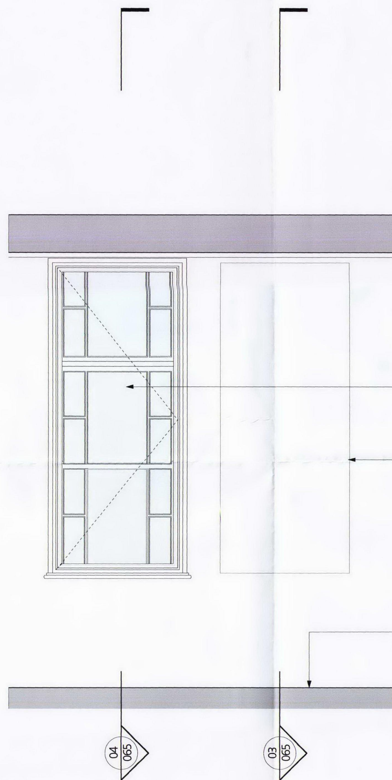
02 Existing Windows Typical Internal Elevation 1:20 @ A1
