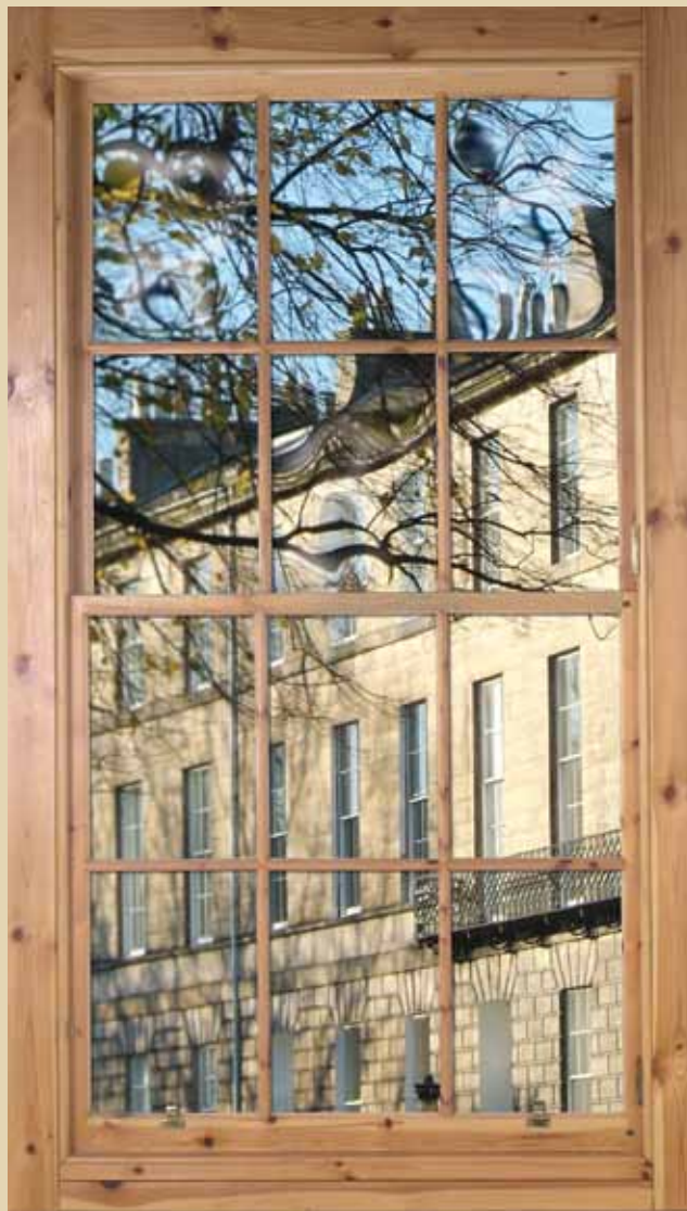
Timber Georgian Sash and Case with Super Slimlite Double Glazed Units with 6mm, 8mm or 10mm cavity will comply with Document L for total overall window U Value 1.6 (See section detail).
