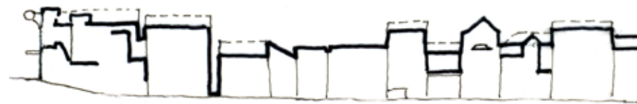
Irregular parapet heights and adhoc roof forms from flat , mono pitched, hipped, gabled and turreted
