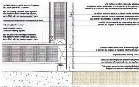
DETAIL DESIGN OF THE ADJUSTABLE BEARING SHOE AND WALL & FLOOR SECTION SCALE 1.5
