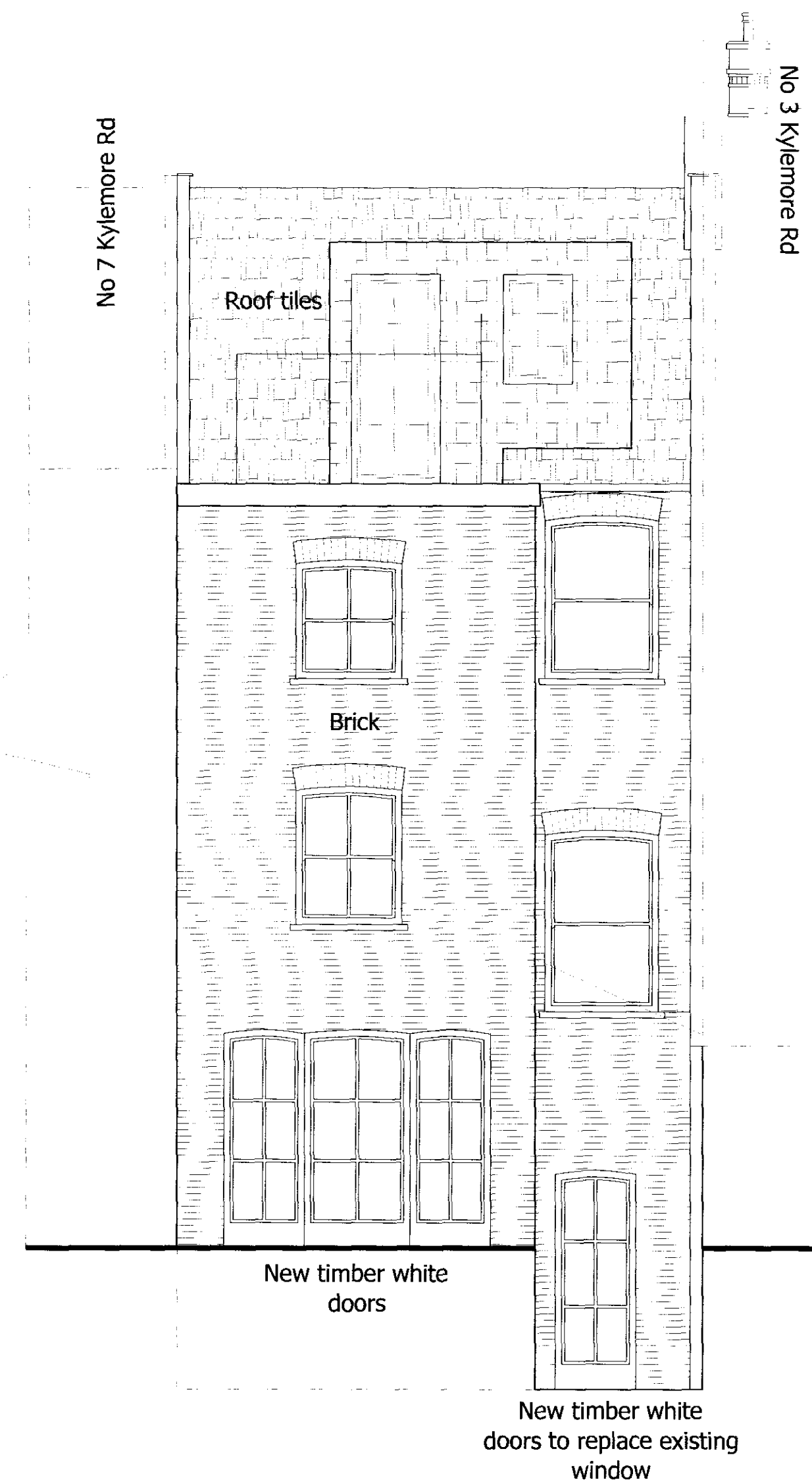
Rear elevation behind proposed side extension
