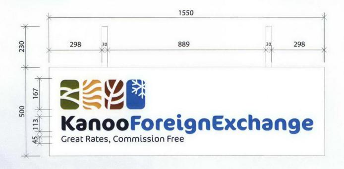
x2 sets of fabricated aluminium sign panels painted white front and back  $1550 \times 500 \times 125$ mm being fret cut with pushed through 10mm thick opal acrylic text and logos with vinyl film to match colours applied to the face (digital printed swatches with matt laminate), strap line in vinyl film. Fluorescent tube illumination. Complete with hanging supports.
