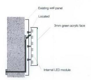
One set off stainless steel build up letters & logo 70mm return with powder coated in green (panton colour ) 10mm rim , green and orange colour translucent vinyl image applied on opal acrylic for Letters and Logo (2 Sections) LED backing with 20mm locator fitting
