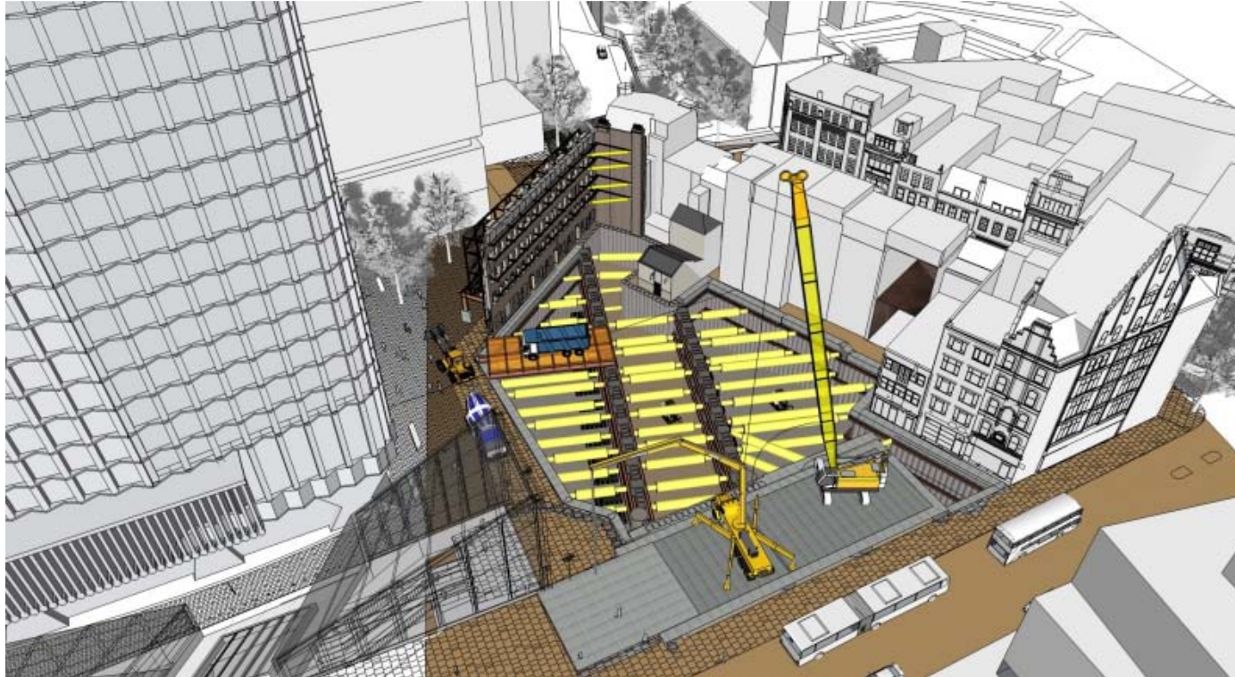
STAGE 21 – CROSS RAIL OVER BASEMENT TEMPORARY PROPPING
