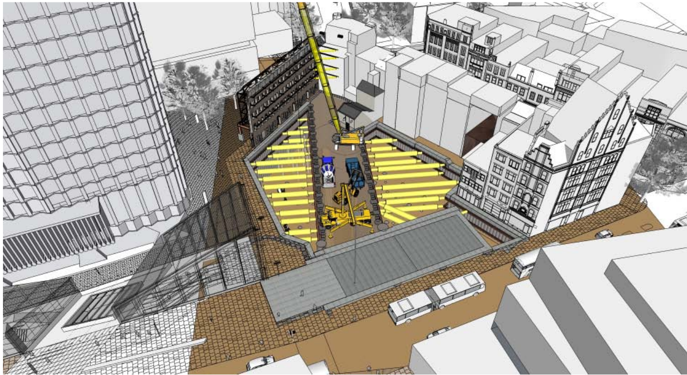
STAGE 14 – NORTHERN BASEMENT EXCAVATION STAGE 2
