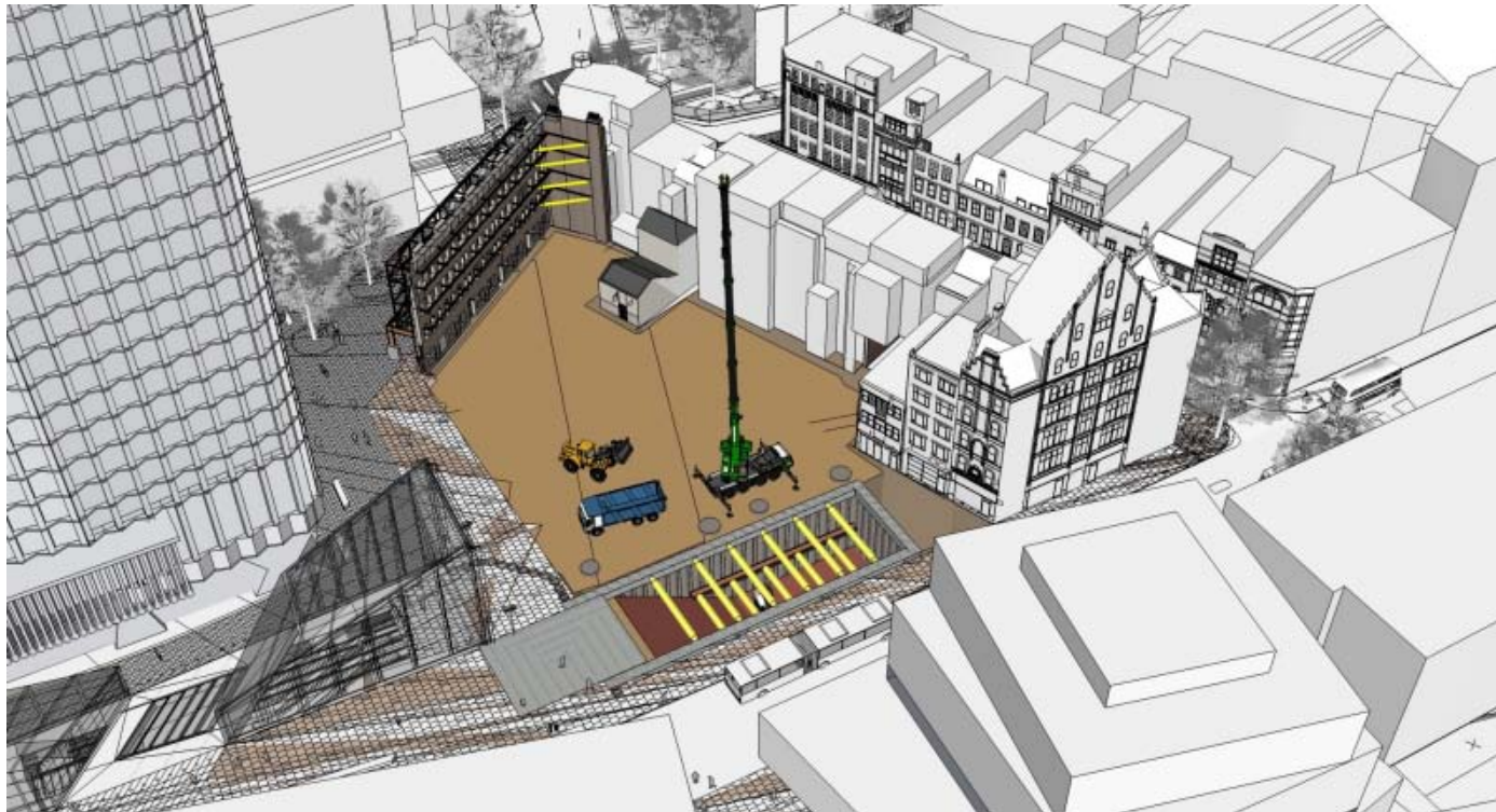
STAGE 6 - LUL ESCALATOR BOX STAGE 3 EXCAVATION
