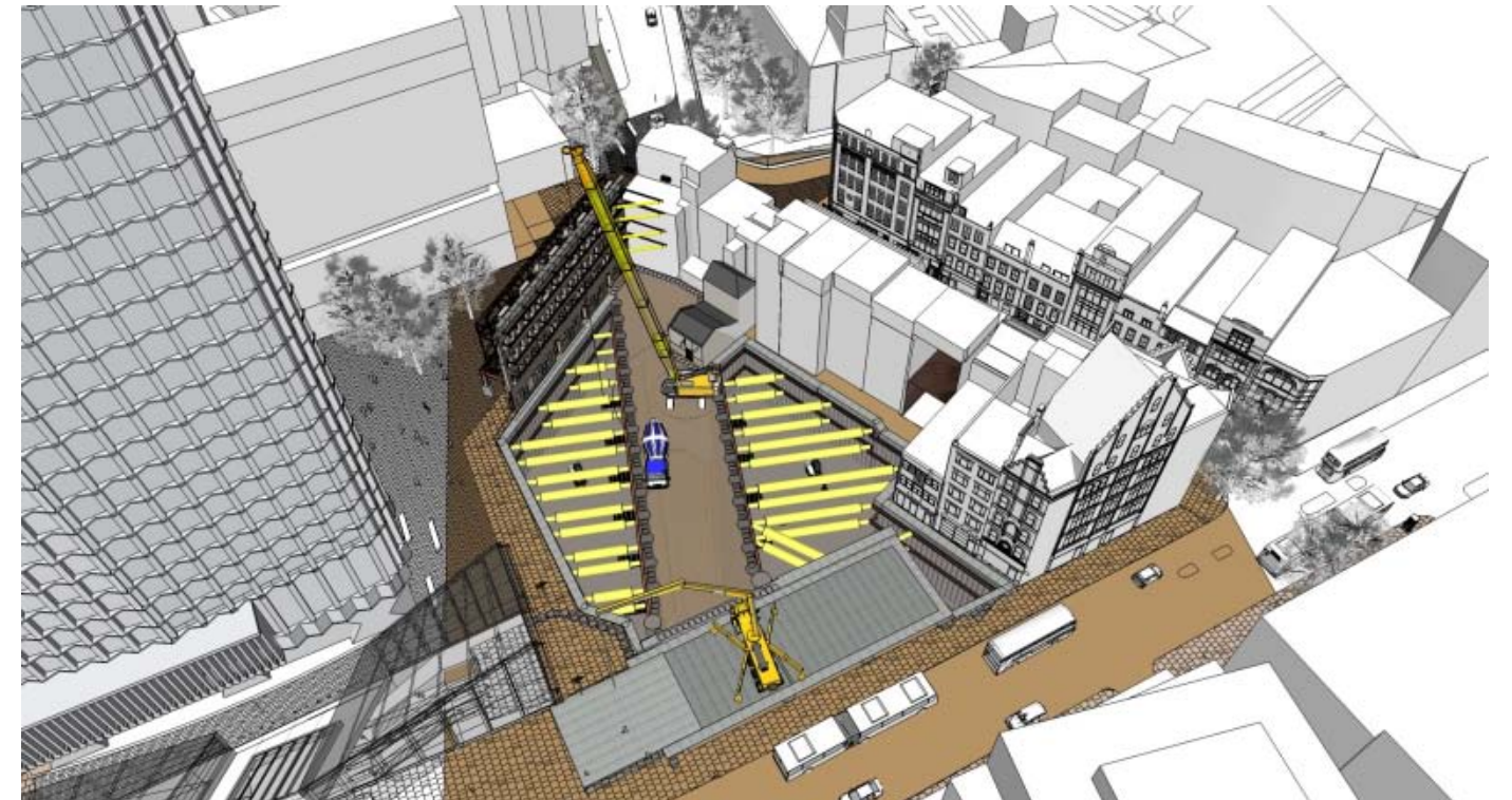
STAGE 16 – SOUTHERN BASEMENT EXCAVATION STAGE 2
