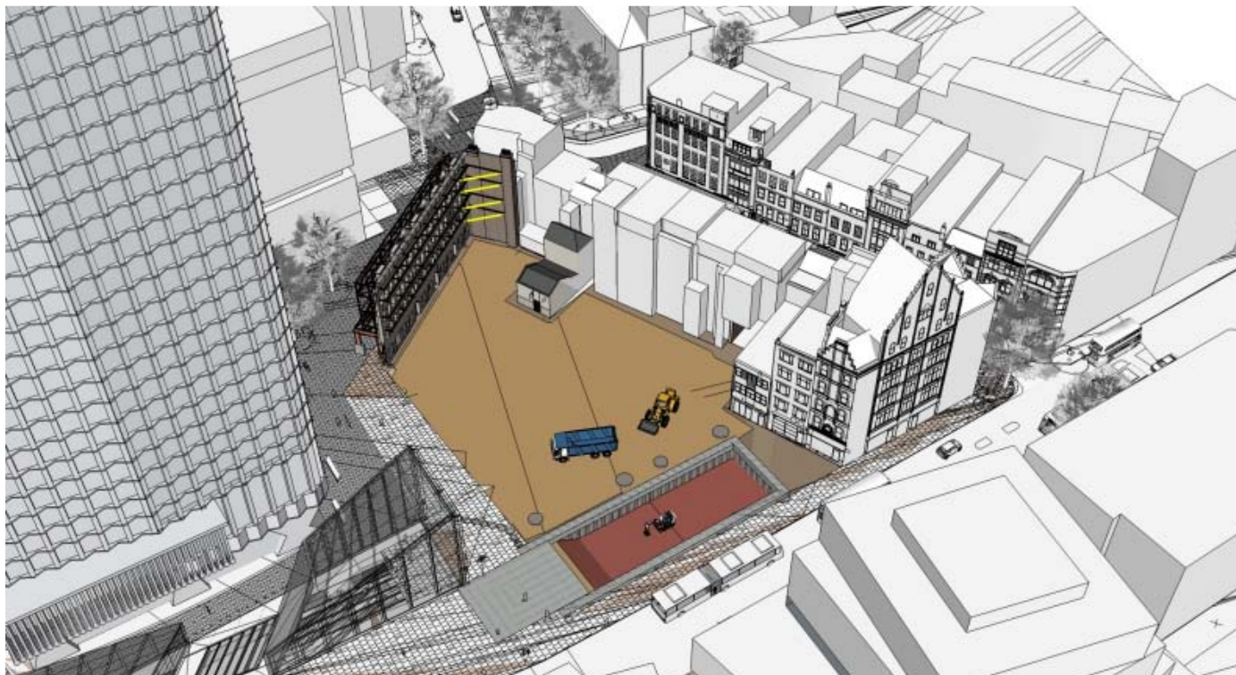
STAGE 2 – LUL ESCALATOR BOX BREAKOUT & STAGE 1 EXCAVATION
