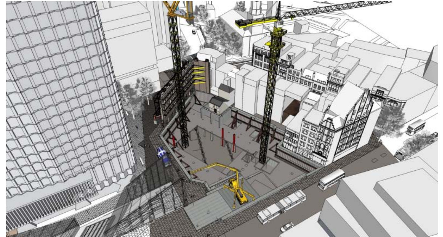
STAGE 27 – CONSTRUCT BASEMENT MEZZANINE SLAB
