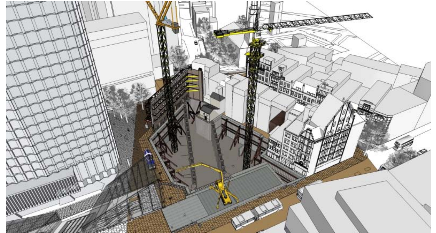
STAGE 24 – REMOVE ALL HORIZONTAL PROPPING SYSTEMS
