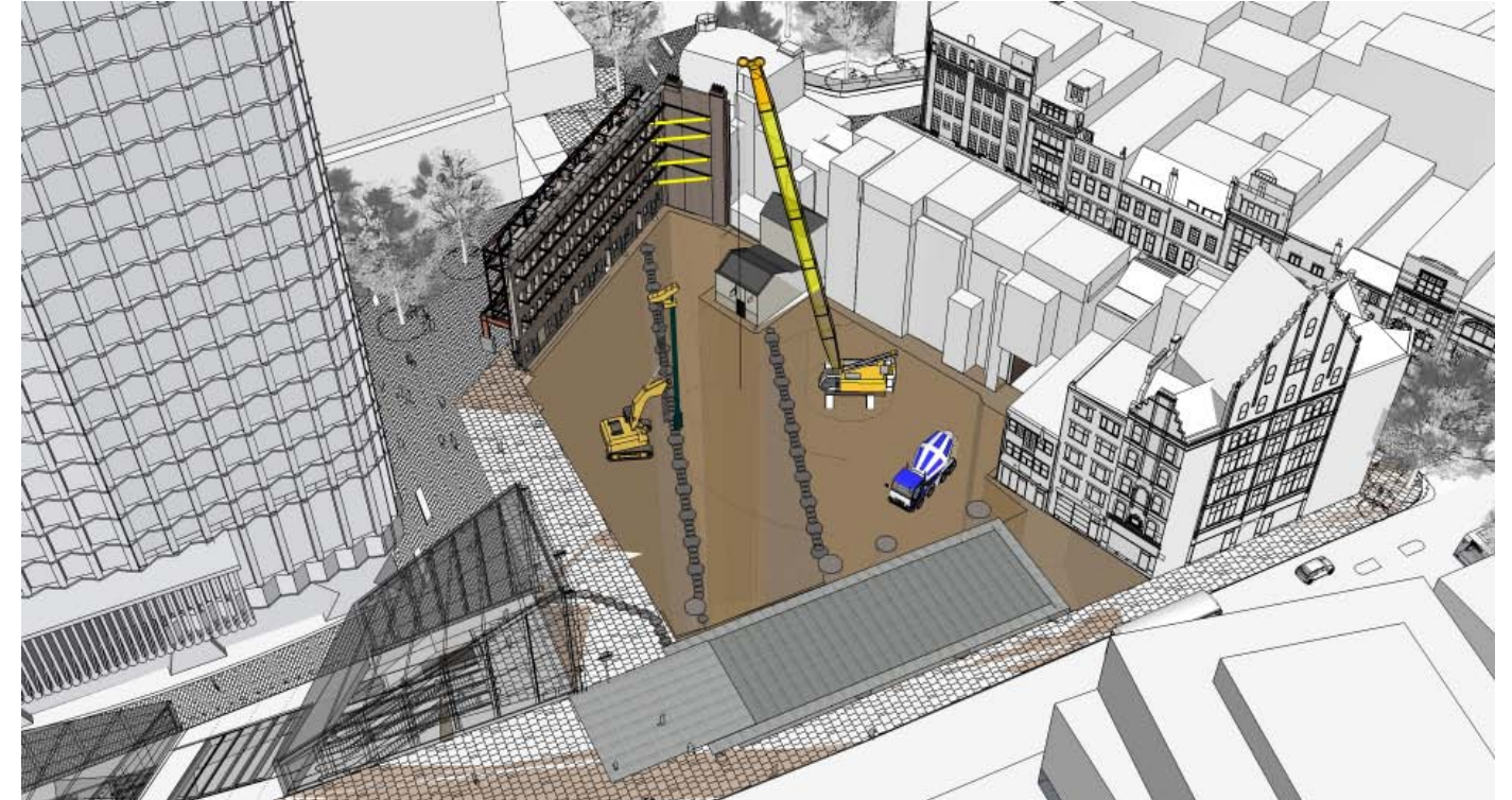
STAGE 7 - PILED WALL CONSTRUCTION TO CROSS RAIL TUNNEL
