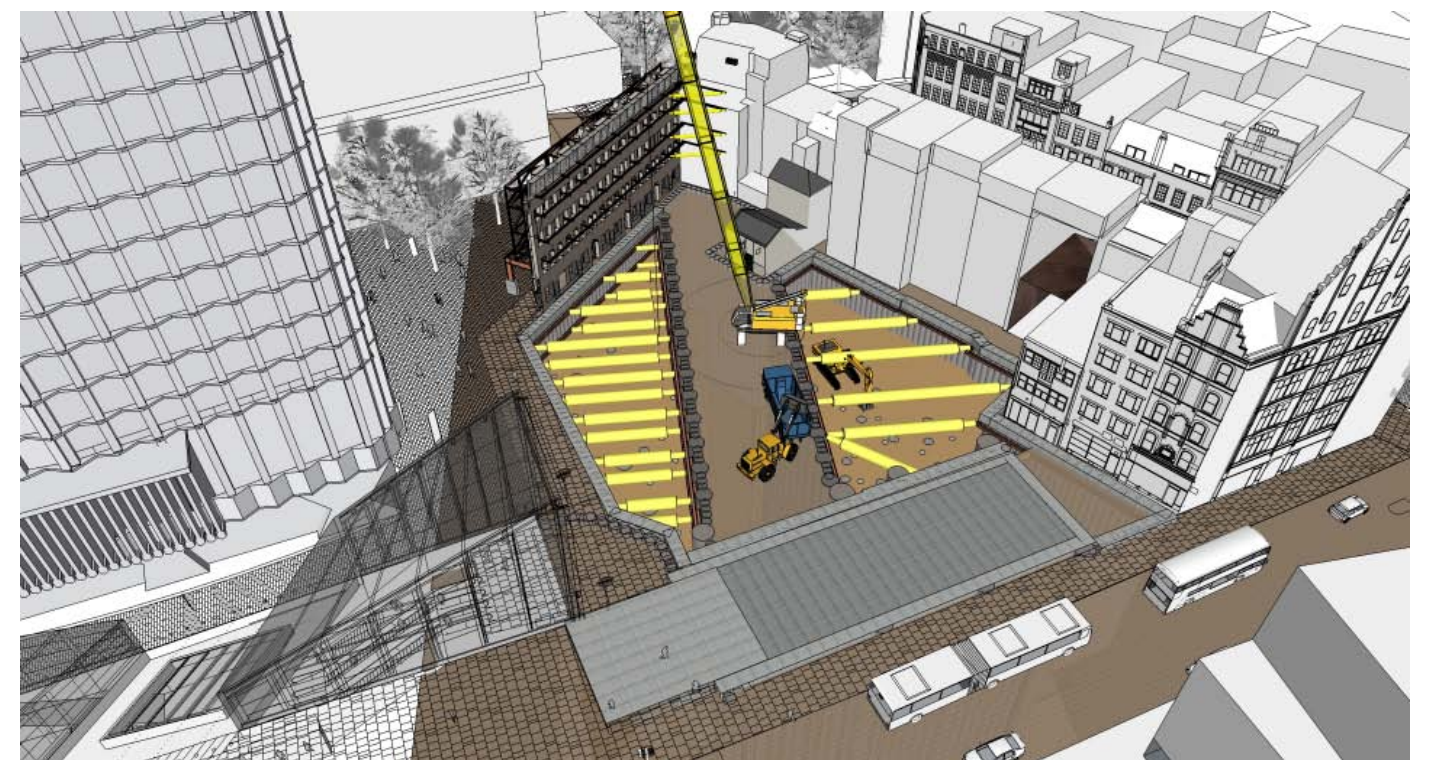
STAGE 12 – EXCAVATION IN SOUTHERN BASEMENT STAGE 1
