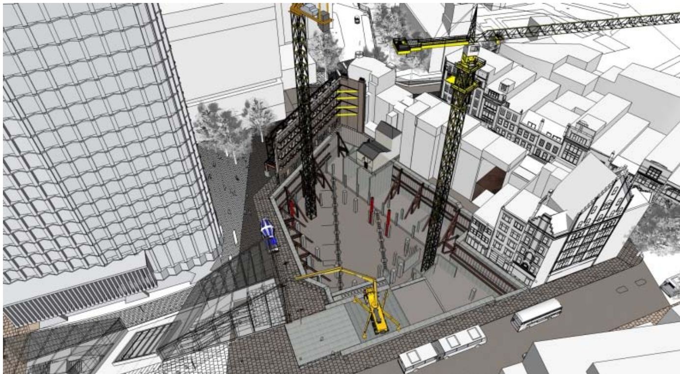
STAGE 26 – CONSTRUCT BASEMENT TO MEZZANINE FLOOR WALLS AND COLUMNS
