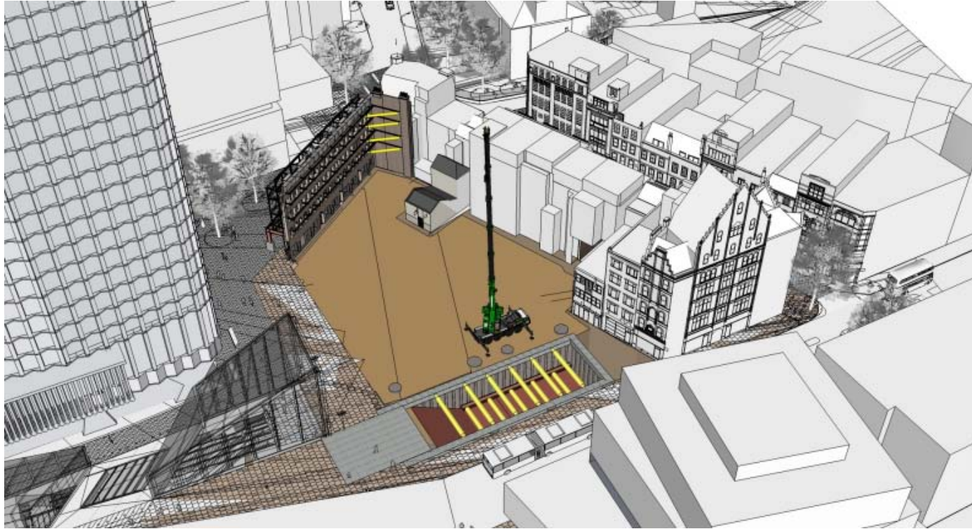
STAGE 5 - LUL ESCALATOR BOX STAGE 2 PROPS INSTALLATION
