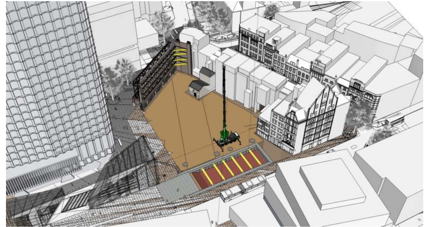
STAGE 3 – LUL ESCALATOR BOX CAPPING BEAM PROPS INSTALLATION
