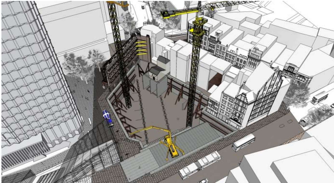
STAGE 25 – DEMOLISH CROSSRAIL TEMPORARY PILES & BREAKOUT LUL BOX
