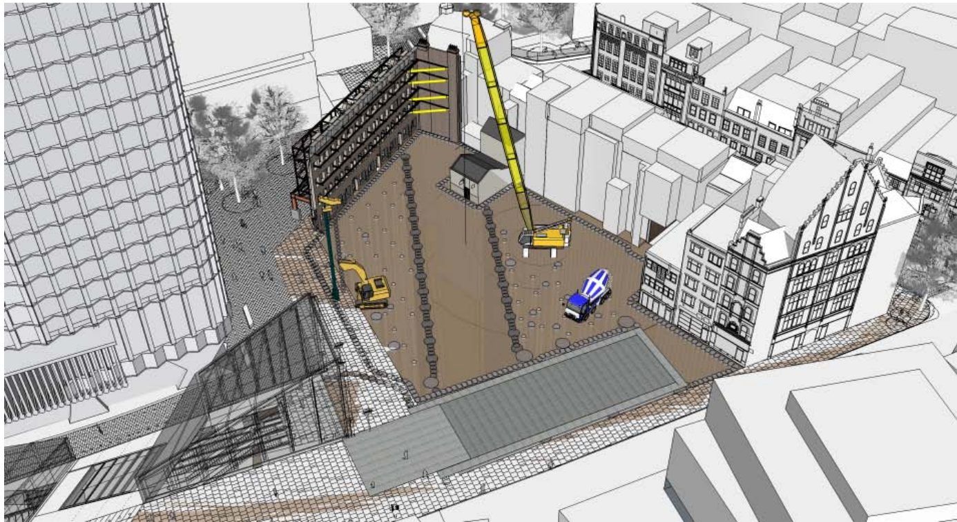
STAGE 9 – MAIN PILES AND TENSION PILES INSTALLATION
