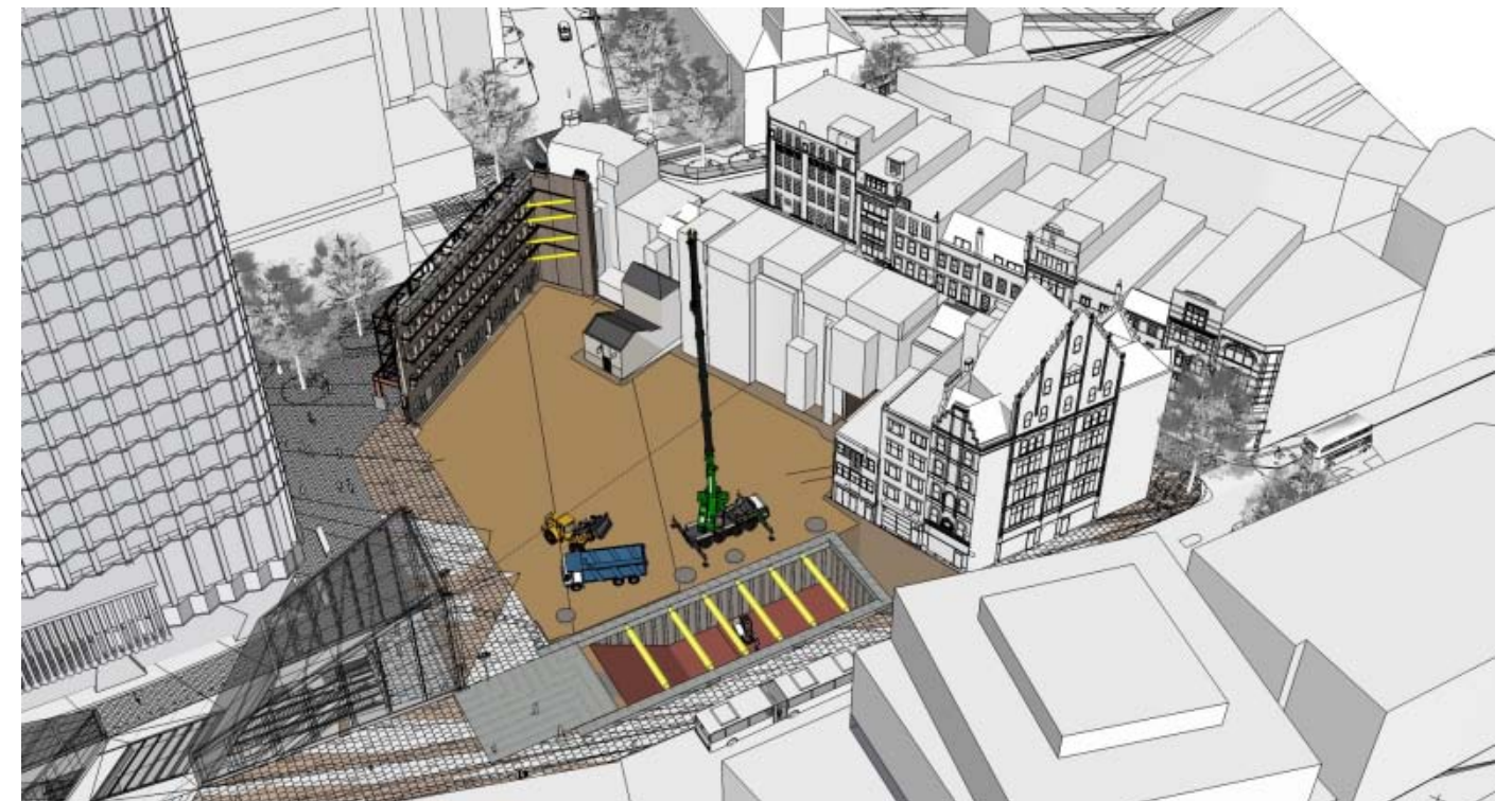
STAGE 4 – LUL ESCALATOR BOX STAGE 2 EXCAVATION
