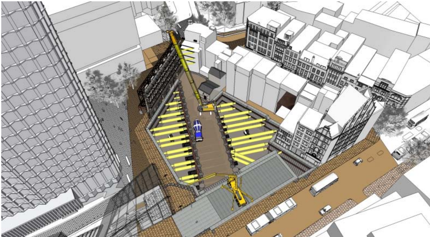
STAGE 17 – ADIT BEAM CONSTRUCTION
