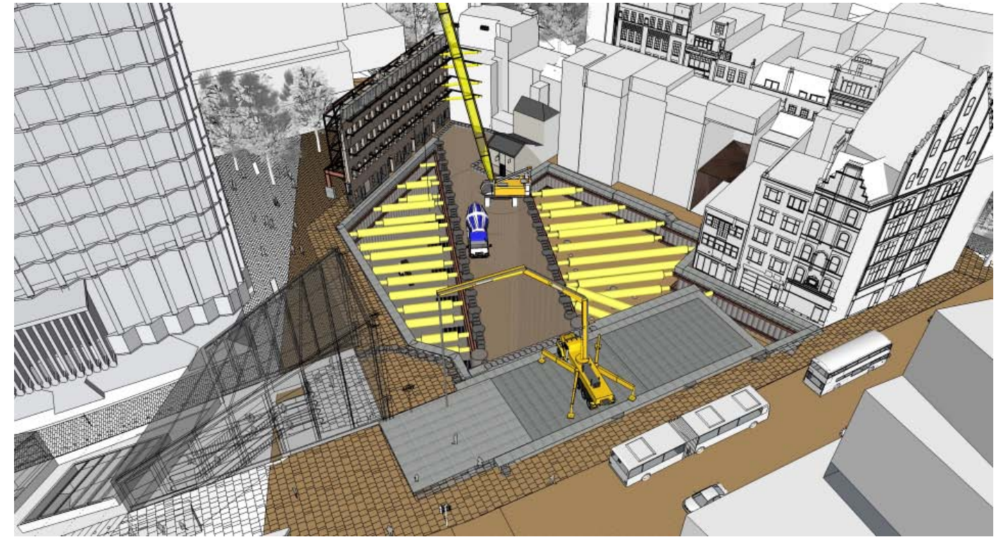
STAGE 15 – NORTHERN BASEMENT SLAB AND ADITS
