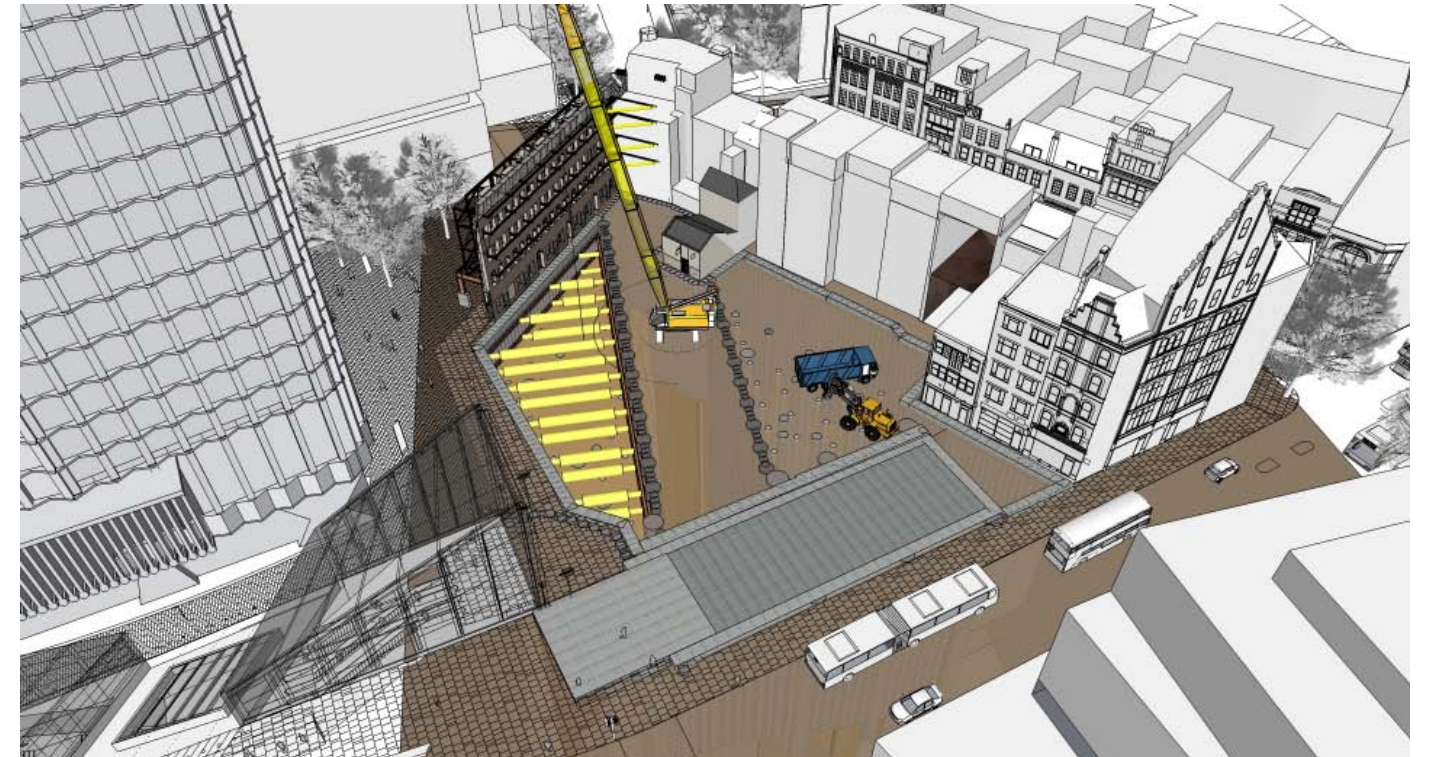
STAGE 11 – INSTALL TEMPORARY PROPS IN NORTHERN BASEMENT
