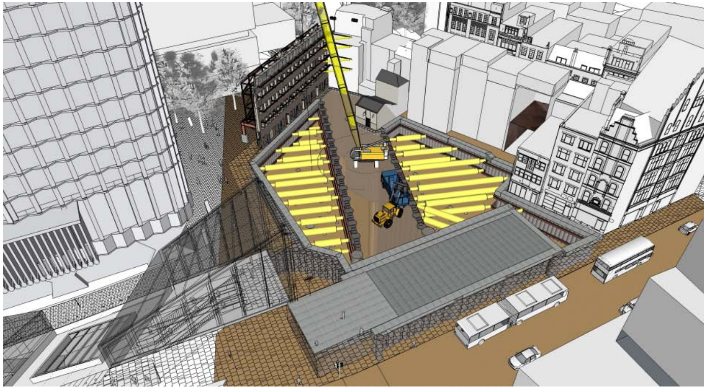
STAGE 13 – INSTALL TEMPORARY PROPPING IN SOUTHERN BASEMENT
