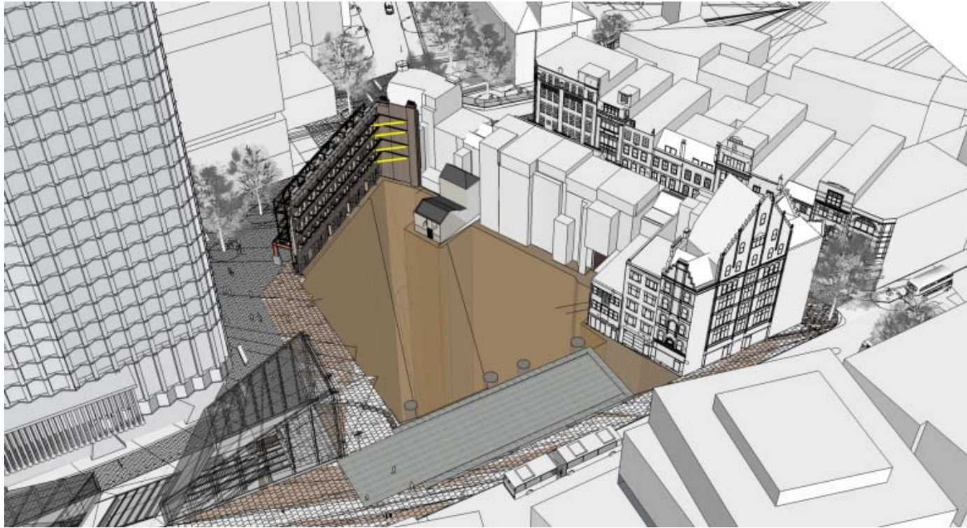
STAGE 1 – DEMOLITION, ENABLING WORKS & FAÇADE RETENTION
