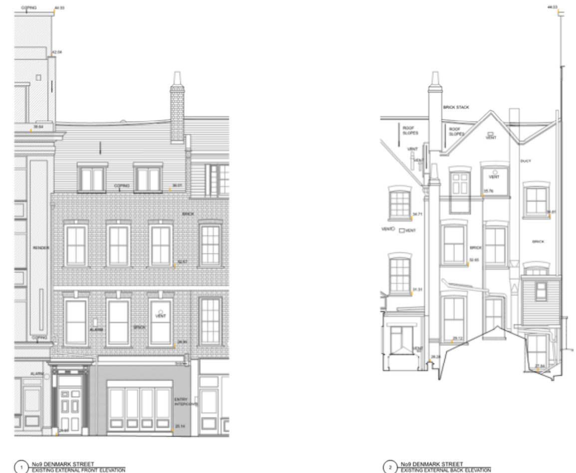
Figure 2.2 Front & Rear Existing Elevations
