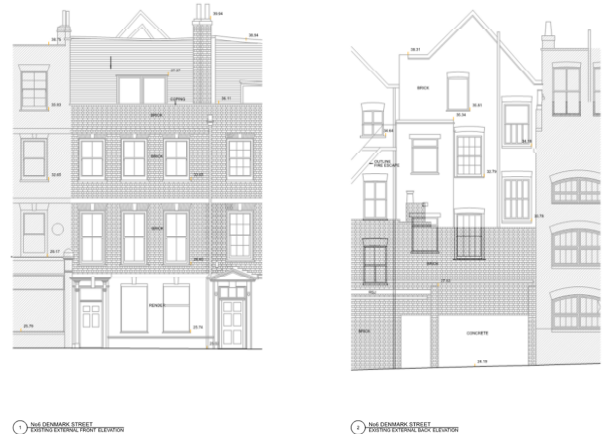
Figure 5.2 Front & Rear Existing Elevations
