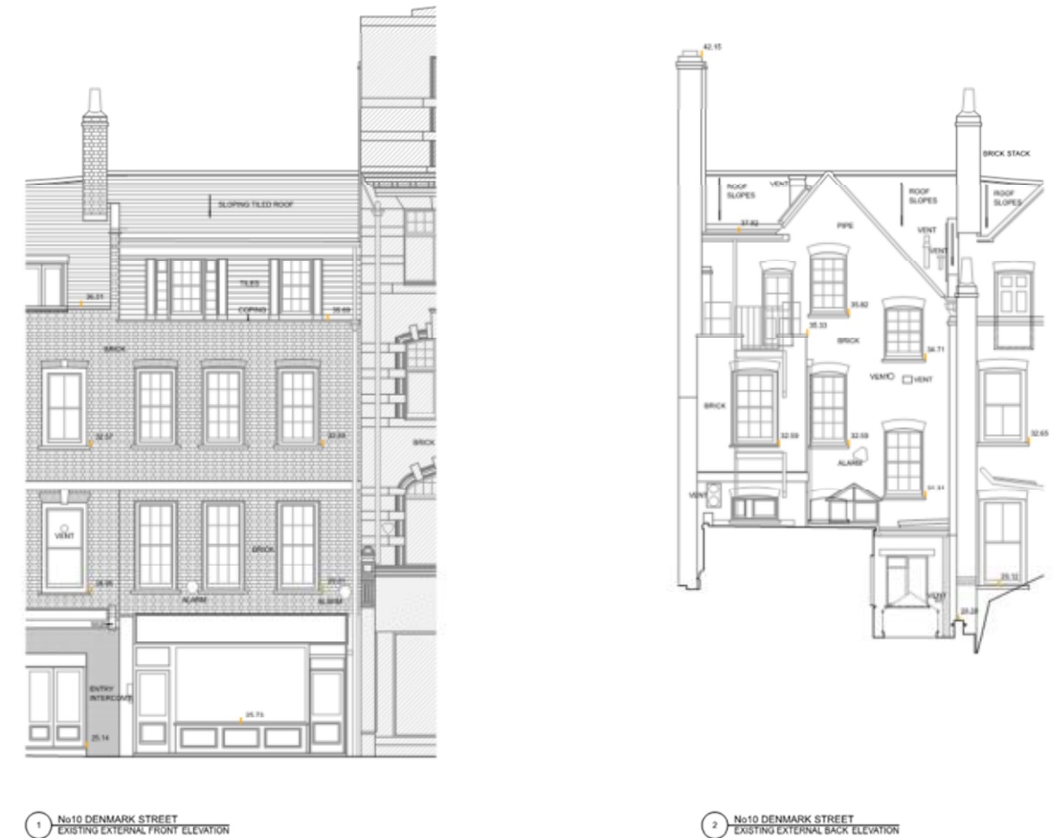
Figure 3.2 Front & Rear Existing Elevations
