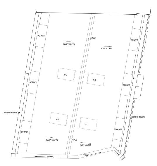
17 No4 FLITCROFT STREET THIRD FLOOR PLANS SHOWING EXTENT OF STRIP OUT 18 No4 FLITCROFT STREET ROOF PLANS SHOWING EXTENT OF STRIP OUT
