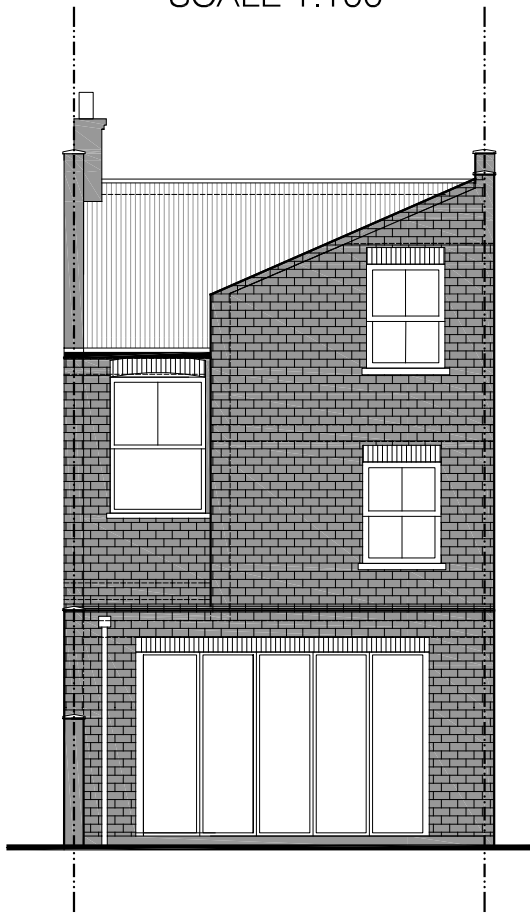
PROPOSED REAR ELEVATION SCALE 1:100
