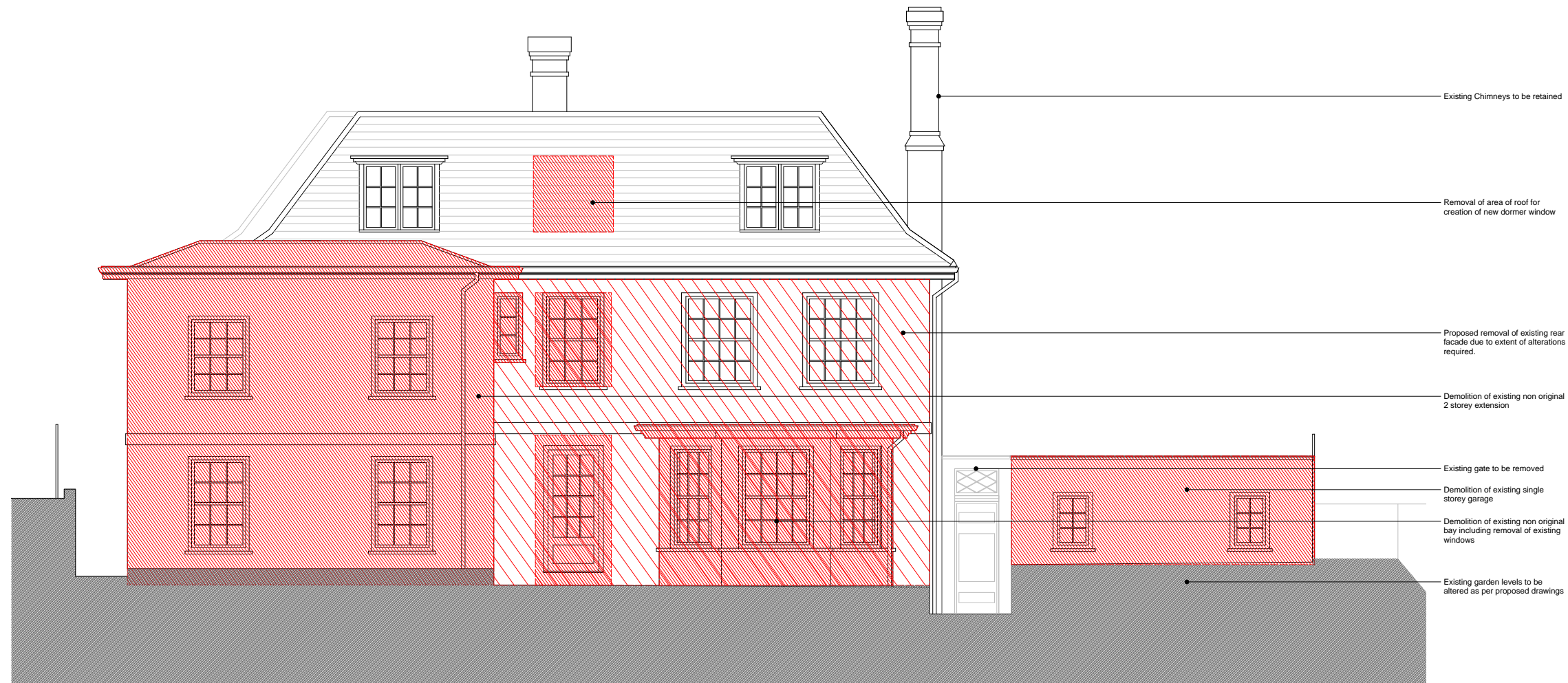
01 Existing Rear Elevation (indicating proposed demolitions)
