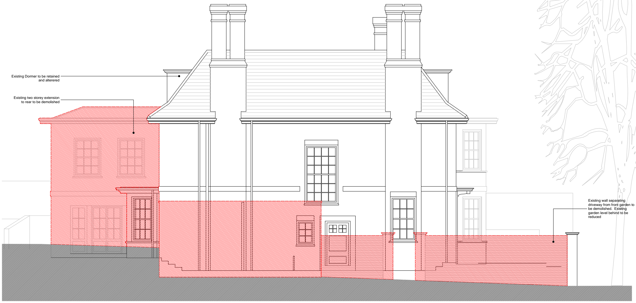
01 Existing Side Elevation (South) (indicating proposed demolitions)
