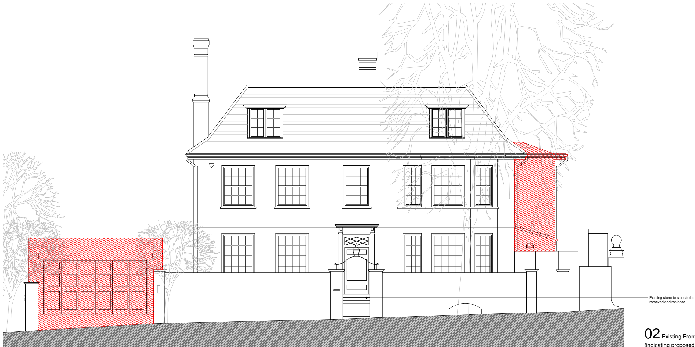
01 Existing Front Elevation (indicating proposed demolitions)
