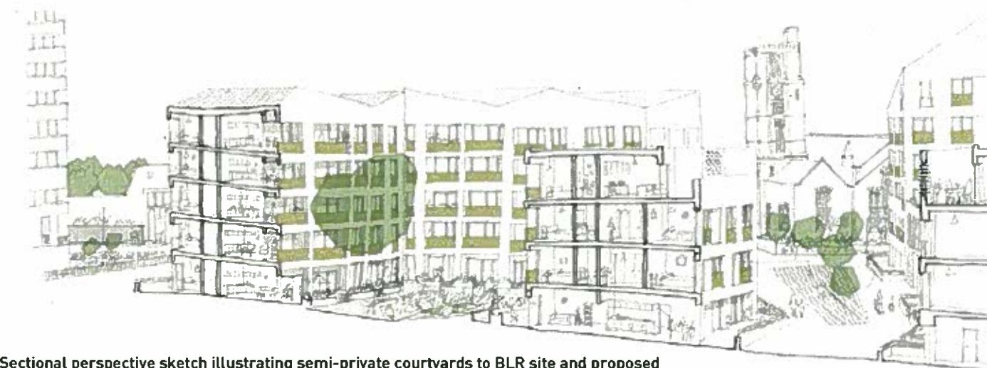
D: Sectional perspective sketch illustrating semi-private courtyards to BLR site and proposed 'New Street' with soft landscaping providing views toward St. Martin's Church
