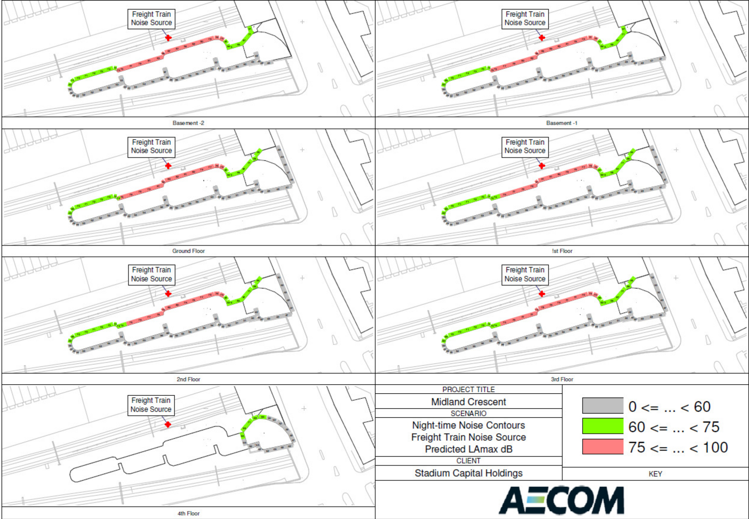
Figure D.4: Night-time L Amax Noise Levels at North Facade
