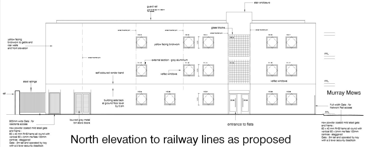
For further materials notes see front elevation; yellow facing brickwork with precast concrete coping velfac windows grey aluminium doors binstore doors green roof, with gunmetal colour aluminium trims
