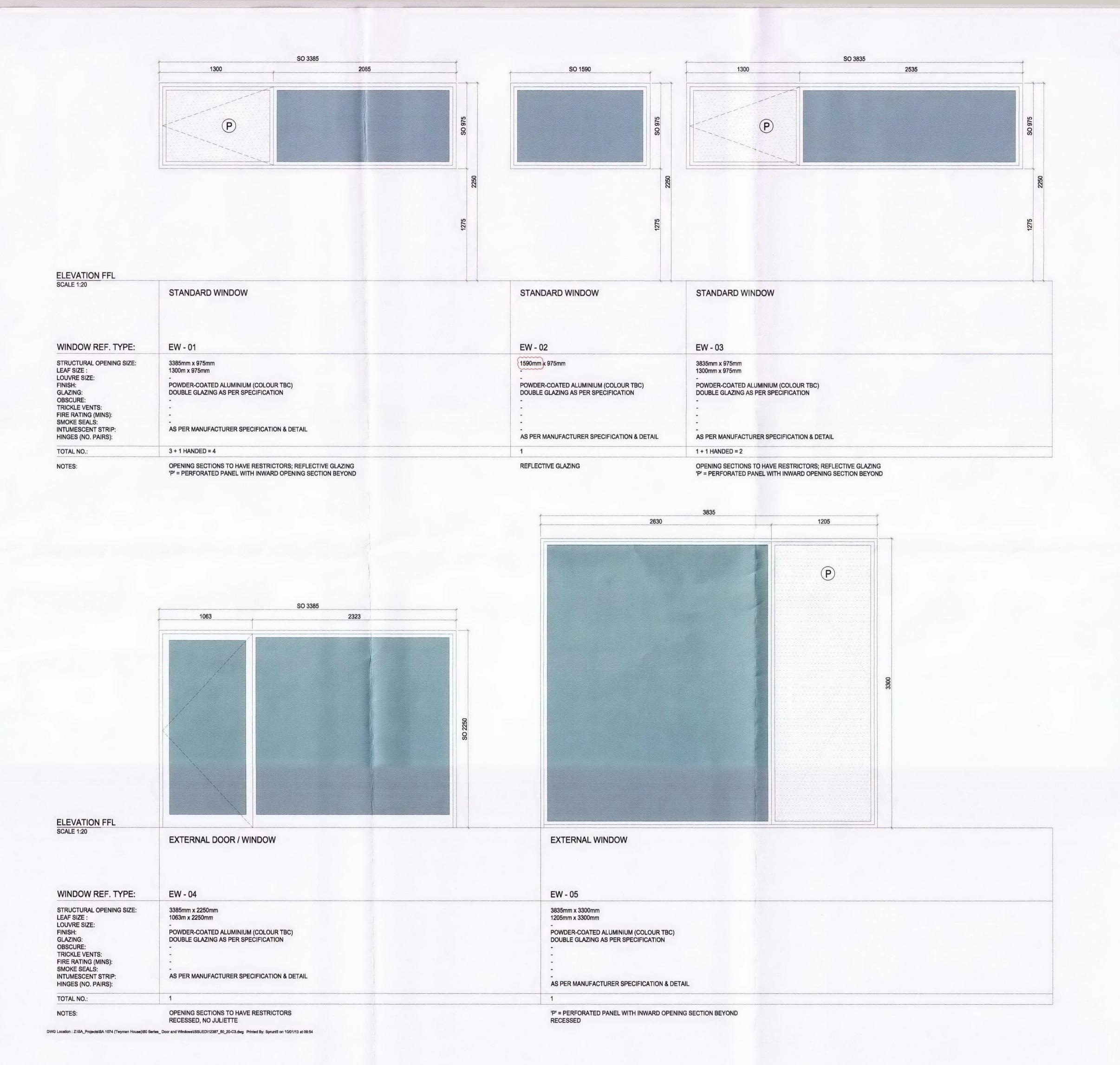
DO NOT SCALE DIMENSIONS OFF THIS DRAWING CHECK ALL DIMENSIONS ON SITE BEFORE FABRICATION REPORT ALL ERRORS OR OMISSIONS TO SPRUNT LIMITED THIS DRAWING IS PROTECTED UNDER COPYRIGHT AND SHALL NOT BE REPRODUCED IN PART OR WHOLE WITHOUT PRIOR EXPRESSED PERMISSION OF SPRUNT LIMITED
