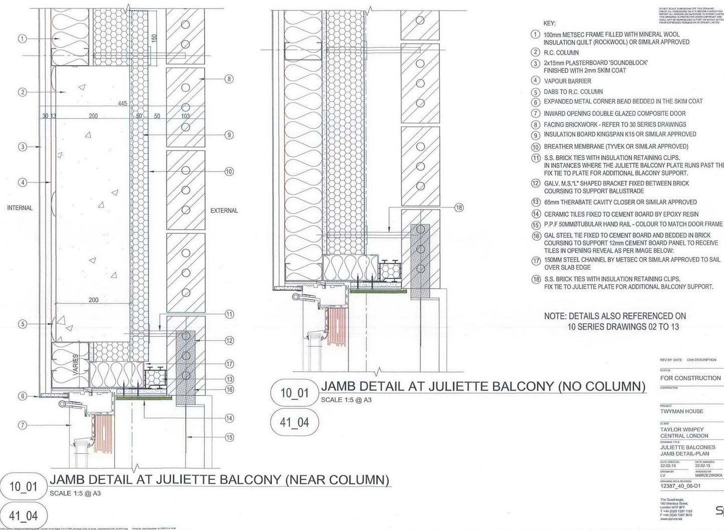
(1) 100mm METSEC FRAME FILLED WITH MINERAL WOOL INSULATION QUILT (ROCKWOOL) OR SIMILAR APPROVED
