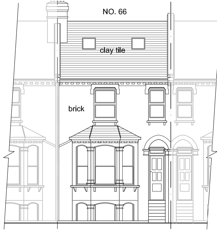
NORTH ELEVATION (FRONT)
