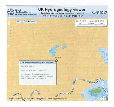
As given in the above image, these soils have essentially no groundwater and, hence, no measurable flows. Indeed, the permeability for natural London Clay is in the order of 3 X 10<sup>-10</sup> metres /second.
