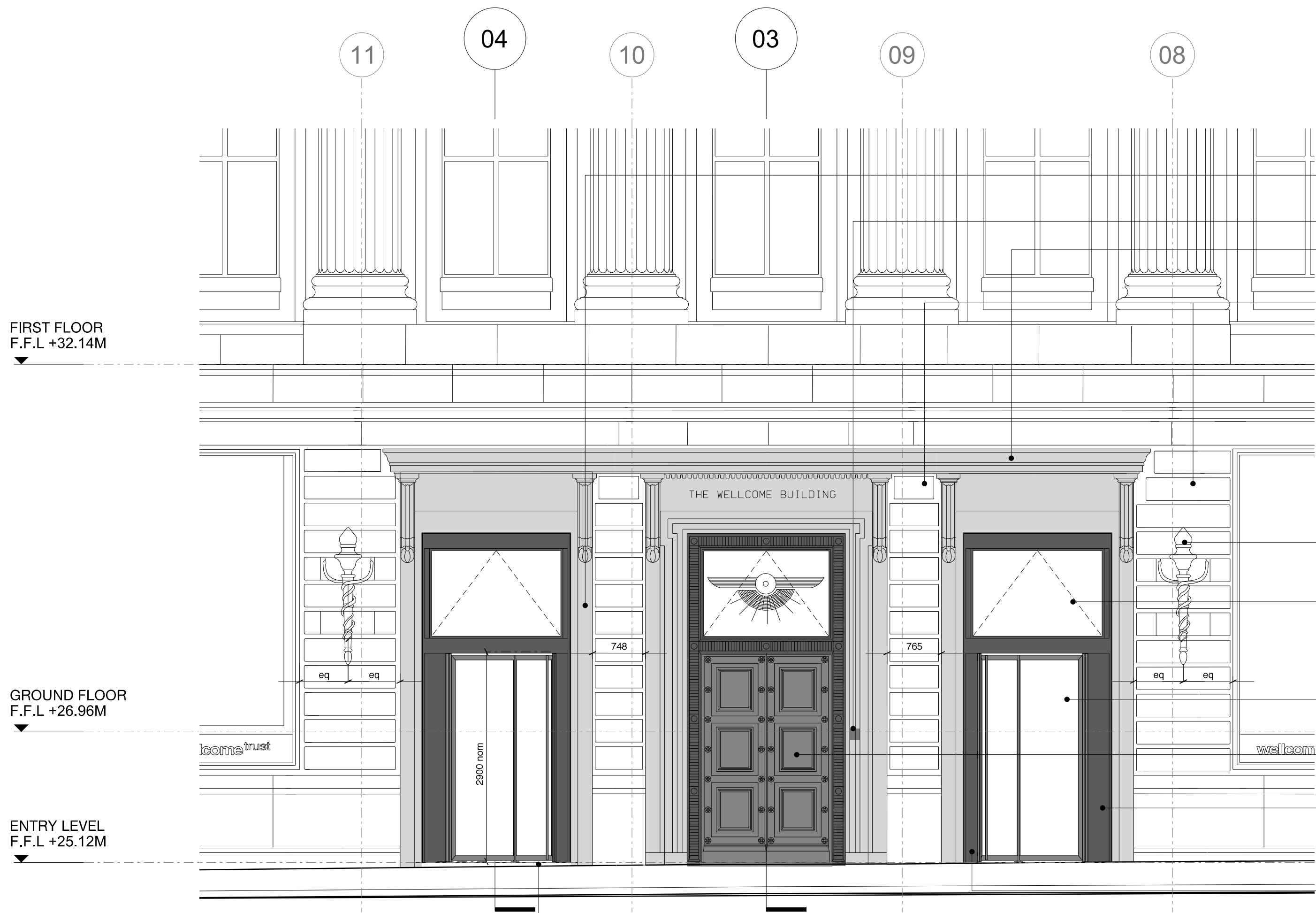
01 MAIN ENTRANCE - NORTH ELEVATION ELEVATION - SCALE 1:50
