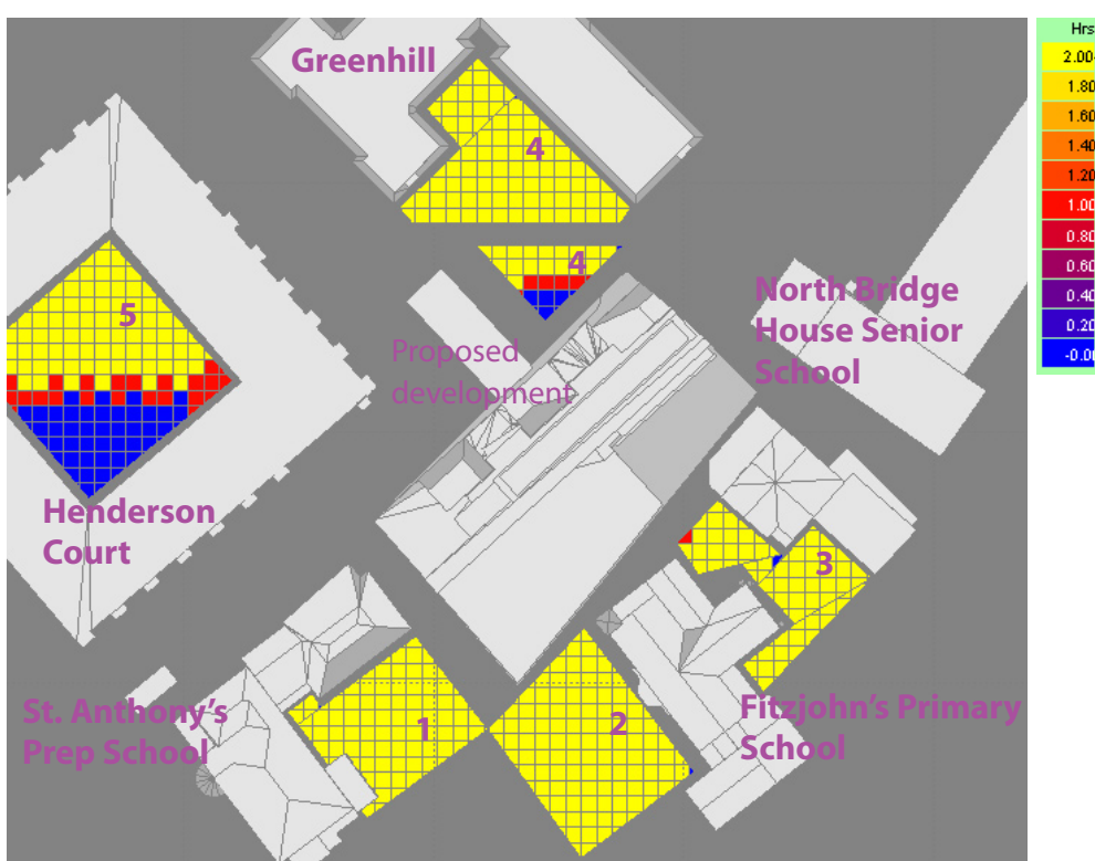
Location of open spaces with the proposed development in place. Yellow indicates that at least 2 hours of sunlight is received.
