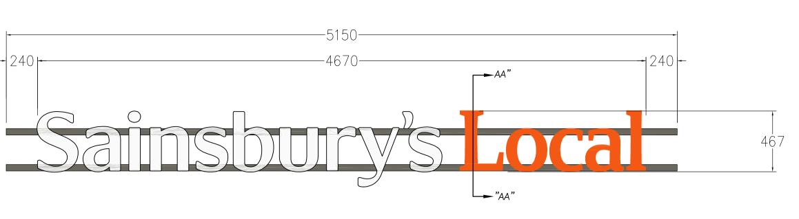
450 HIGH (CAPITALS) INTERNALLY ILLUMINATED CANISTER LETTERING, 'SAINSBURY'S' IN WHITE, 'LOCAL' IN ORANGE, APPLIED TO POWDER-COATED STEEL RAILS - QUARTZ GREY RAL 7039; ILLUMINATION BY LOW VOLTAGE LED FITTINGS - WHITE = 98 CANDELAS/m², ORANGE = 48 CANDELAS/m².
