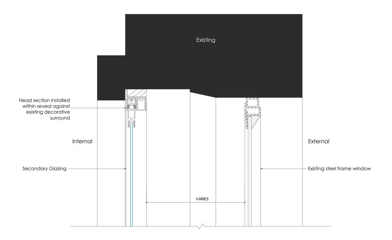
Typical secondary glazing head detail 1:2 @ A1
