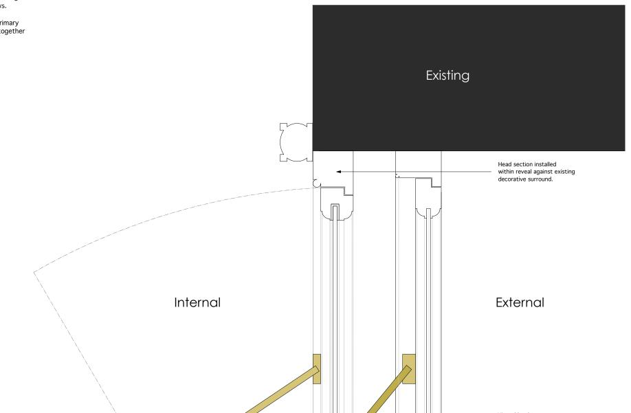
Typical secondary glazing head detail 1:2 @ A1
