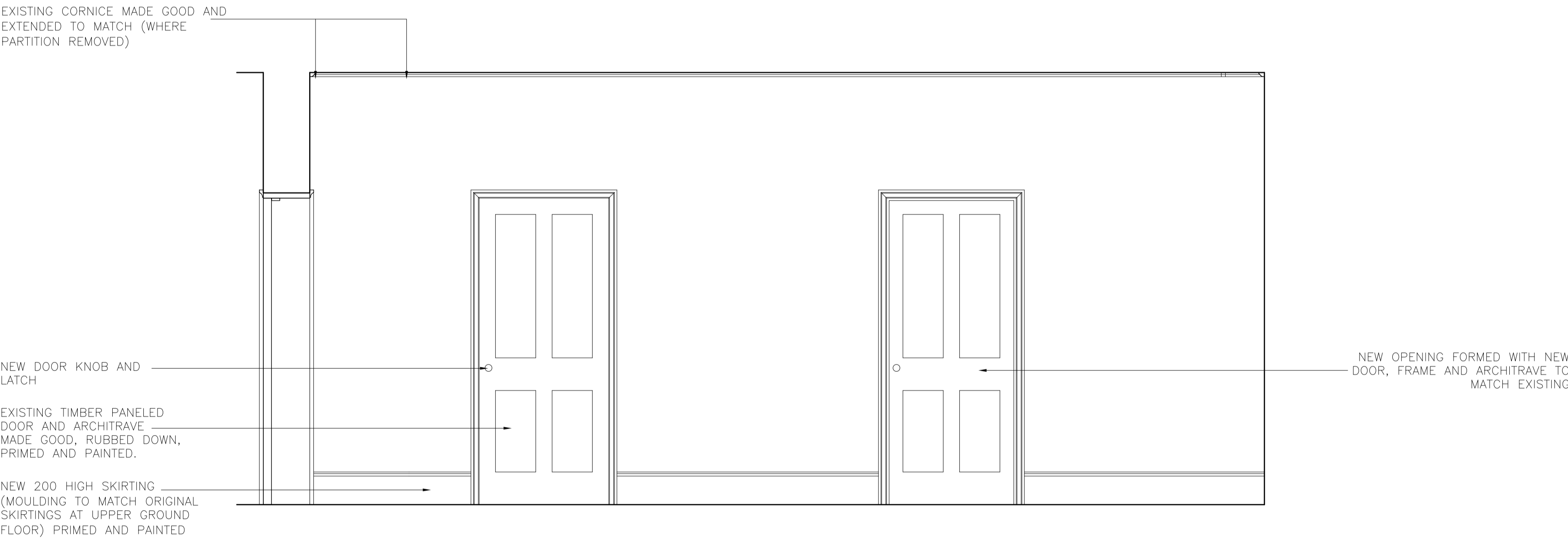
PROPOSED INTERNAL ELEVATION 1
