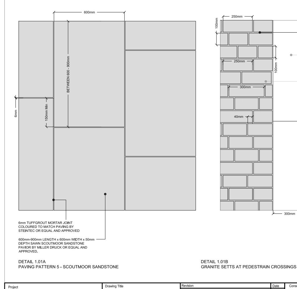
10-15mm TUFFGROUT JOINT COLOURED TO MATCH PAVING BY STEINTEC OR EQUAL AND APPROVED
