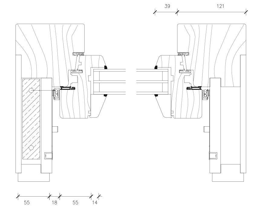
Bayer triple-glazed timber frame sliding sash window U-value of 0.81 W/m<sup>2</sup>K
