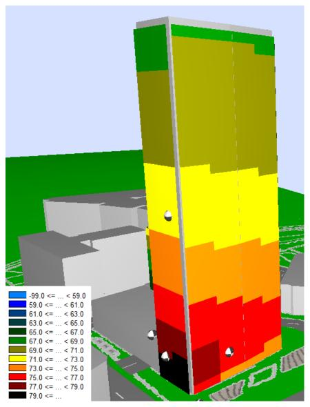
Figure 4 Predicted noise levels: West facade Centre Point Tower
