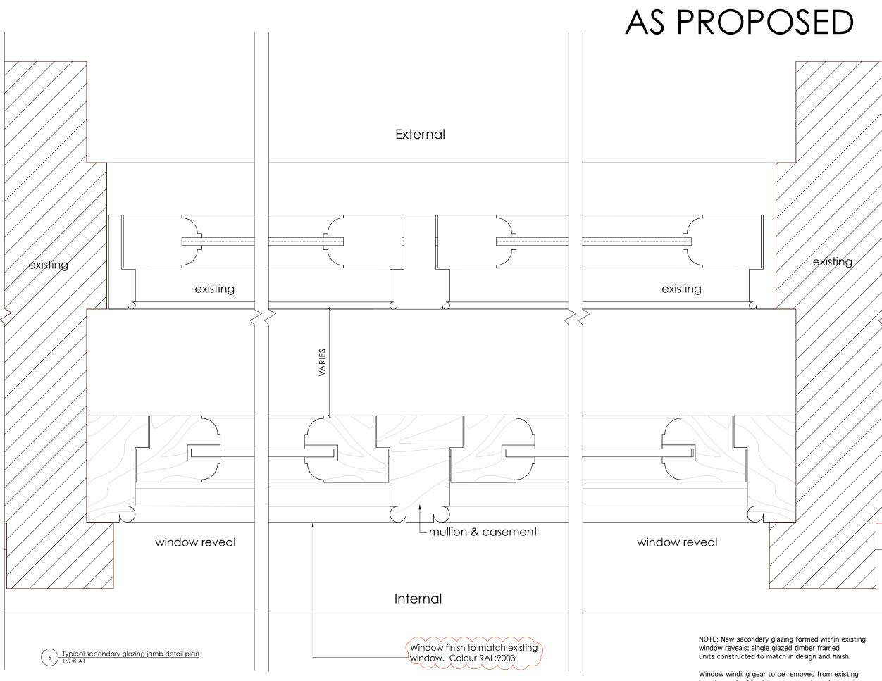
maintain look and feel of existing windows. Hinged bar fixed between secondary & primary glazing fan lights to allow both to open together (as per existing design)
