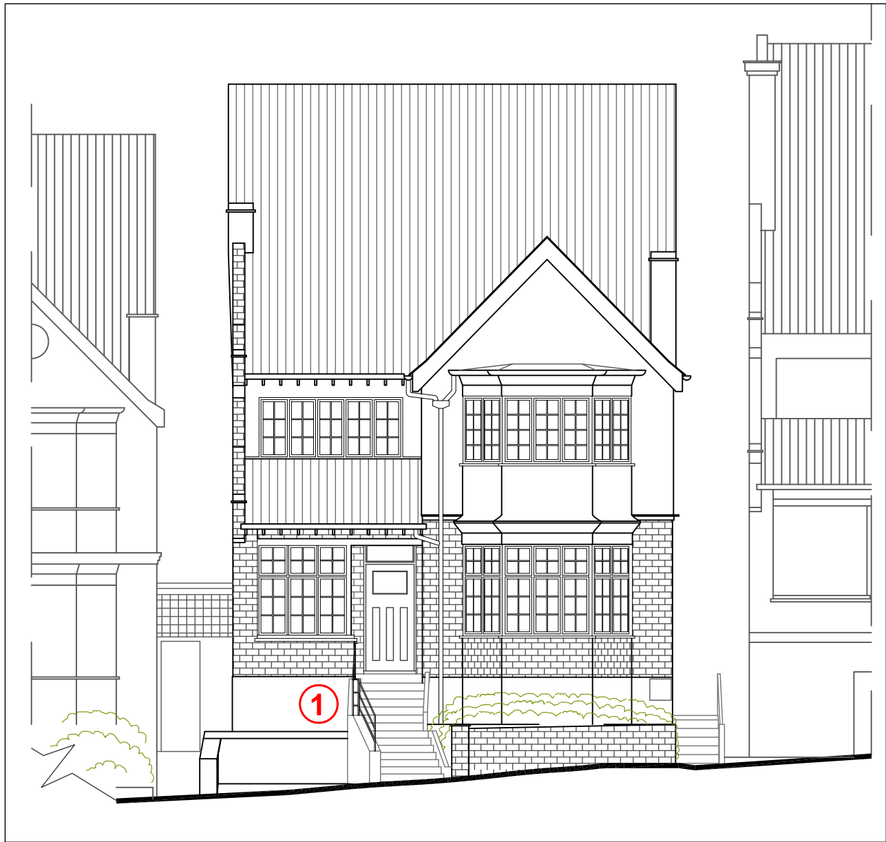
EXISTING STEPS AND SINGLE HANDRAIL
