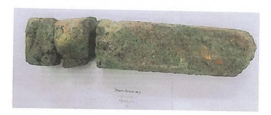
Comments: Material Fair but poorly compacted, Unable to test for compressive strength
