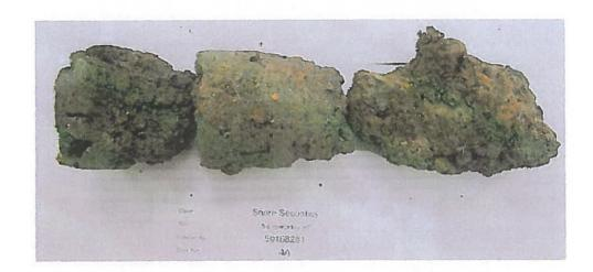
Comments: Material Extremely poorly compacted, Unable to test for compressive strength
