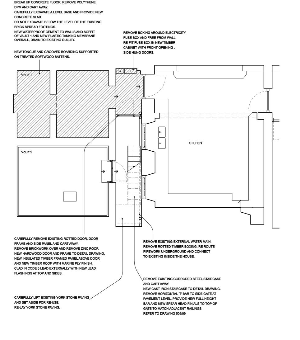
CAREFULLY REMOVE EXISTING SAND/CEMENT RENDER AND MAT REINFORCEMENT FROM WALLS AND SOFFIT
